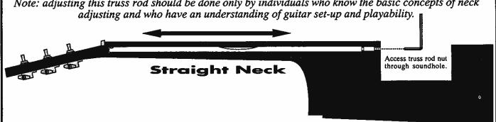
Adjustment is made by inserting a 5 millimeter allen wrench into the silver truss rod nut (through the soundhole), and then turning the nut 1/4 turn for each adjustment until the desired amount of bow (or relief) is reached. Remember: a silver truss rod nut indicates a 2-way truss rod, a brass nut indicates the traditional 1-way truss rod.
