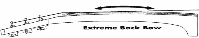
To compensate for an extreme back bow in the neck, turn the truss rod nut COUNTER-CLOCKWISE to move the neck forward into the same direction as the string tension.
